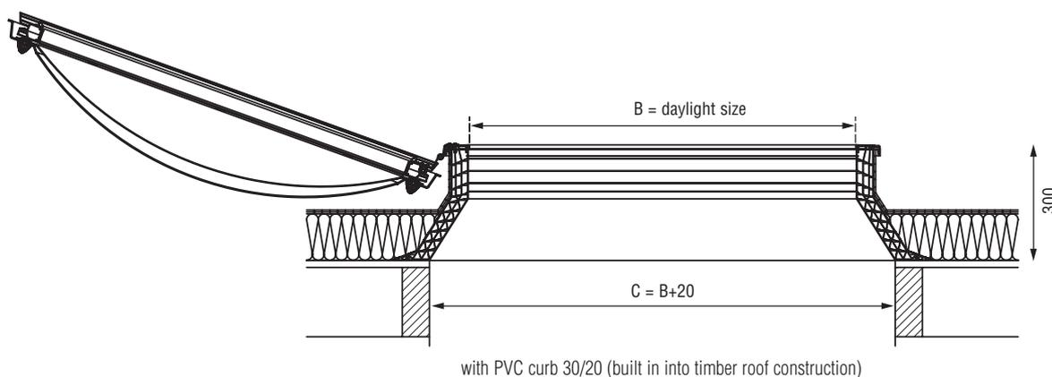
with PVC curb 30/20 (built in into timber roof construction)
